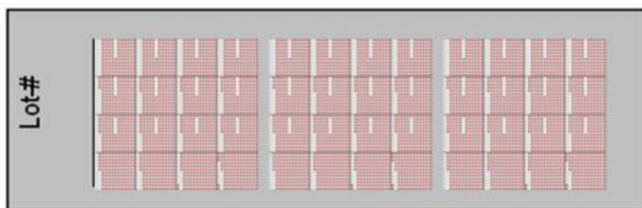
figure 1: schematic view of peptide microarray (3 subarrays; red features indicate individual peptides)
