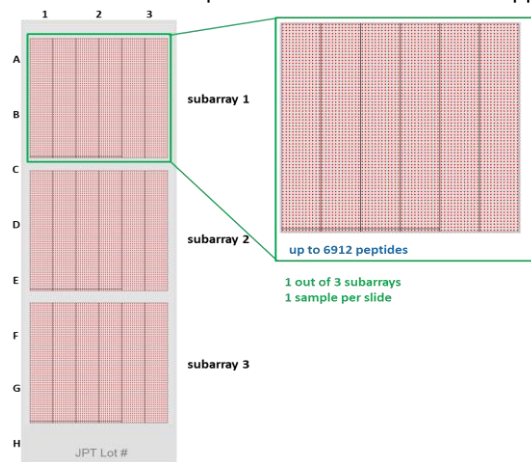
figure 1: Standard array format: Microarray displays all peptides in triplicates (1 spot per subarray)
