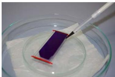
*Capillary forces will suck the solution in between the two slides. Avoid air bubbles within the sandwich.*
